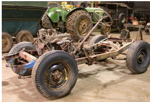
Body off frame, beginning restoration.
